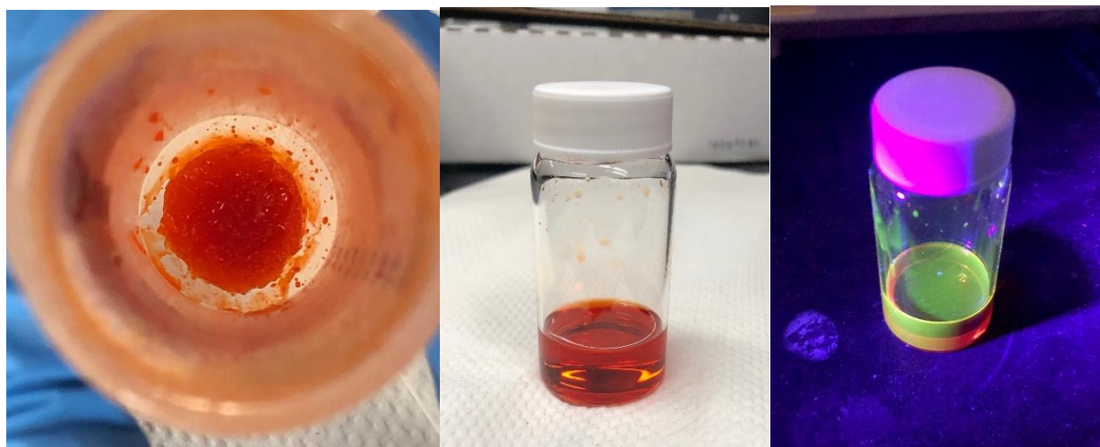
Figure 6.2: From left to right, the purified quantum dots after the final cycle of centrifuging, the QD resuspension in dichloromethane, and the QD-DCM solution under UV light.
